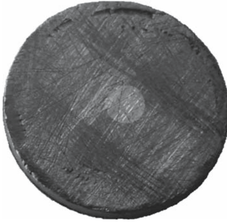
Fig. 2. Demonstrator specimen made of stainless steel with a silver insert of 2 mm diameter. Diameter of the specimen is 12.5 mm.
